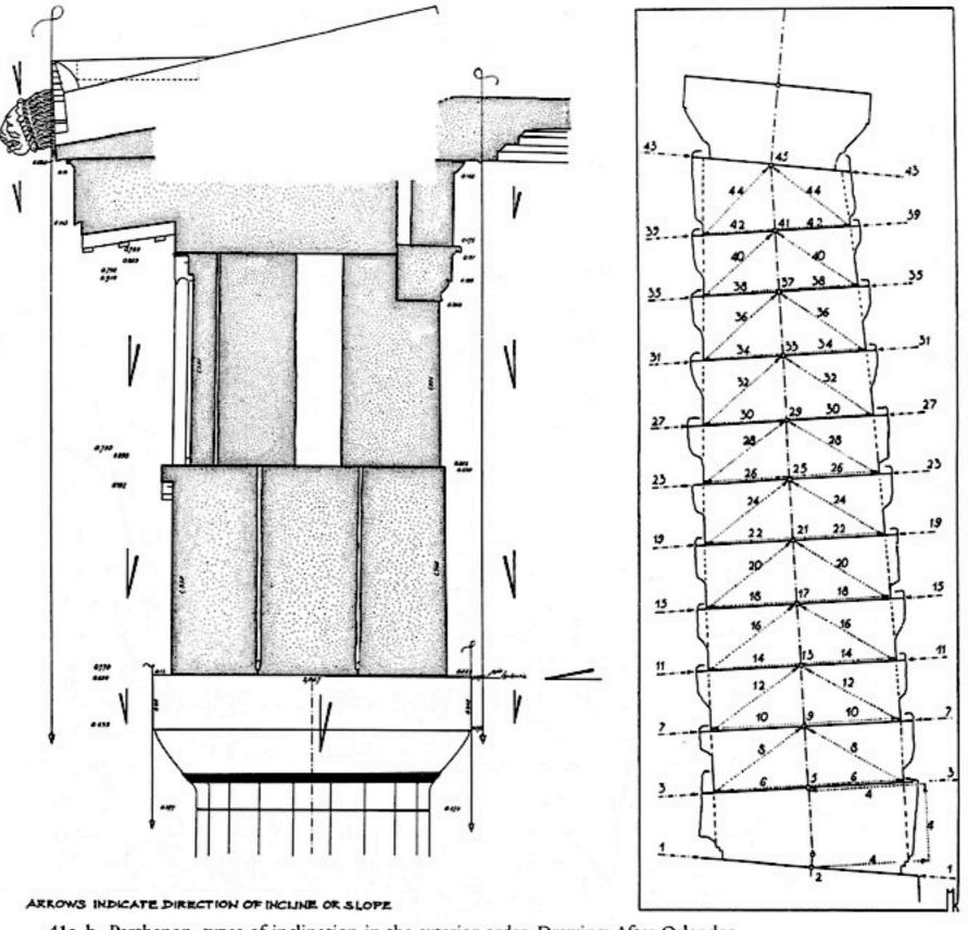
41a-b. Parthenon, types of inclination in the exterior order. Drawing: After Orlandos 1976-77, altered (left) and Korres 1996, 39 fig., detail, altered (right).
