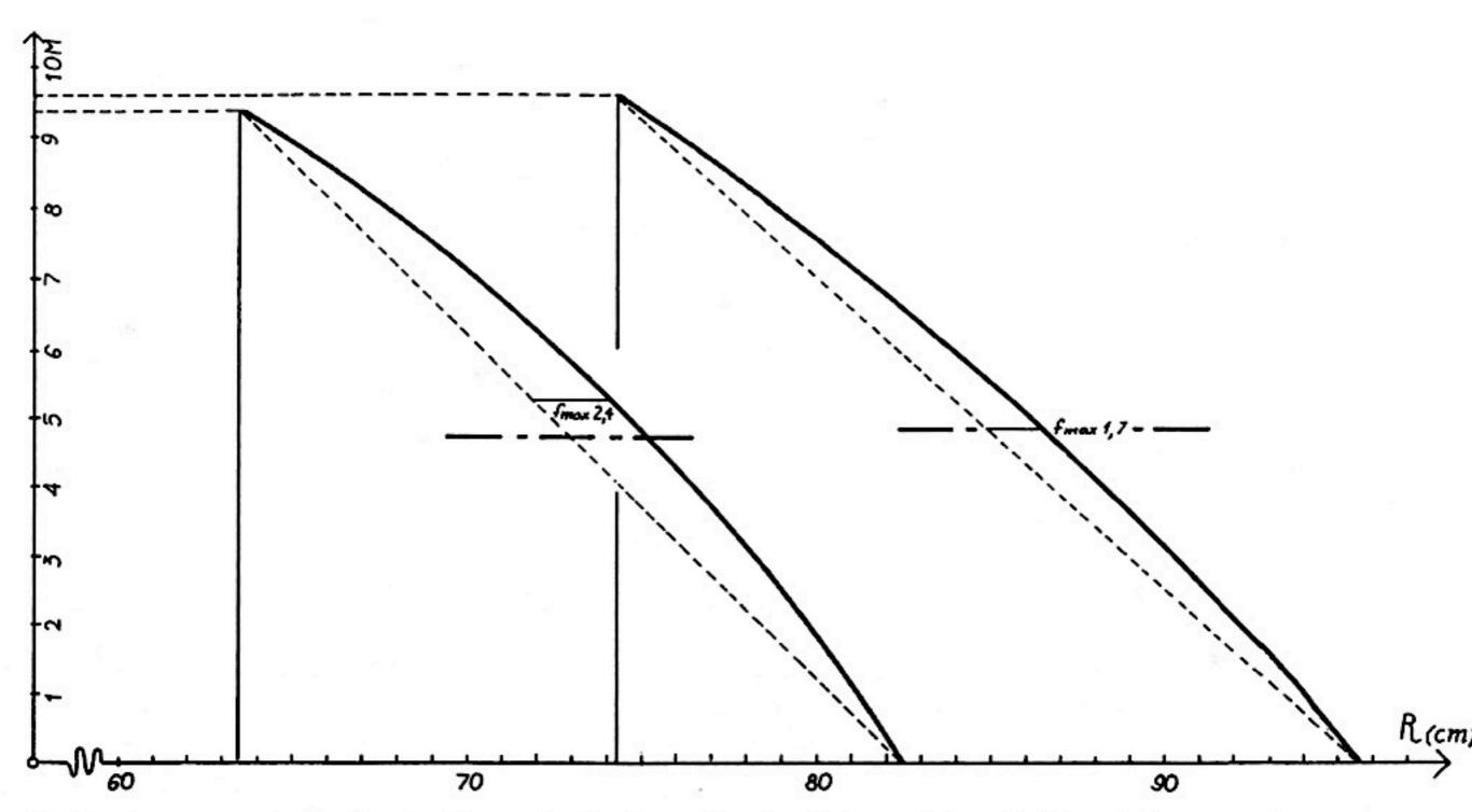
40. Parthenon, entasis of varied intensity in the columns of the pronaos (left) and the peristasis (right), in exaggerated scale. Drawing: After Korres 1999, 96 fig. 3.22, slightly altered.
